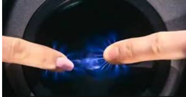
Figure 2. Corona discharge (pattern of light) resulting from the Kirlian effect in high-voltage electro-photography.
